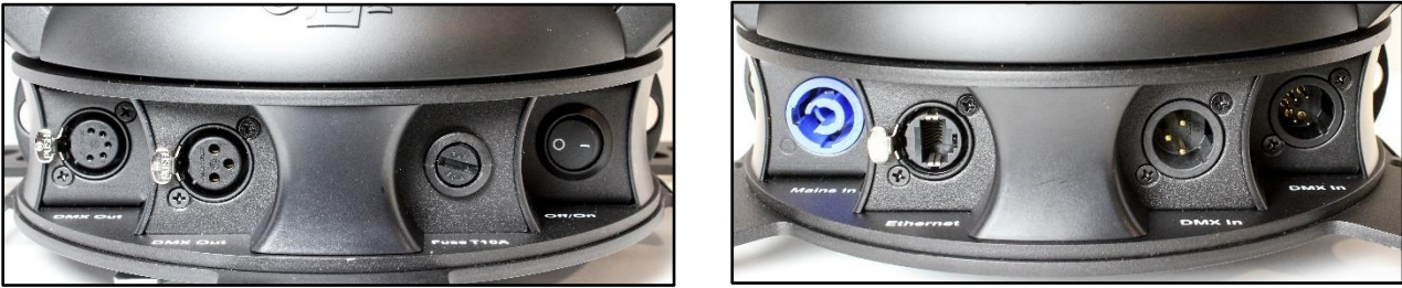
Figure 3-5: GT-1 connection sockets
